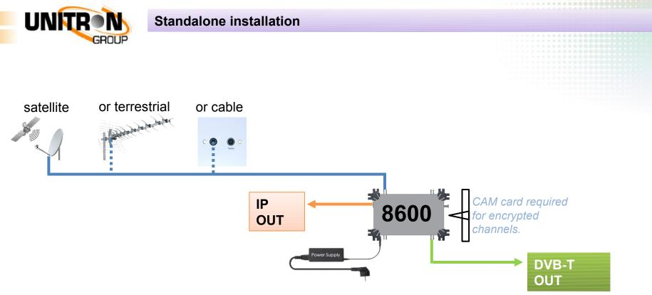
The power supply powers the transmodulator and the LNB or antenna amplifier.
