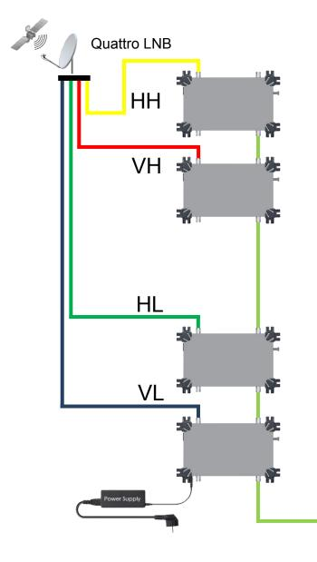
The consumption of the complete setting is too high for 1 power supply.
