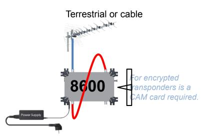
Possiblity to add the converted DVB-T signal to the existing DVB-T signals. The wire must be DC blocked.
